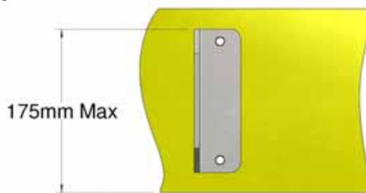
Figure 3, Top Bracket Positioning
