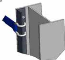
Steel angle on H-beam, internal
